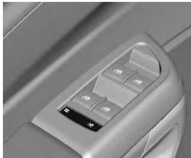
Pressione o interruptor
